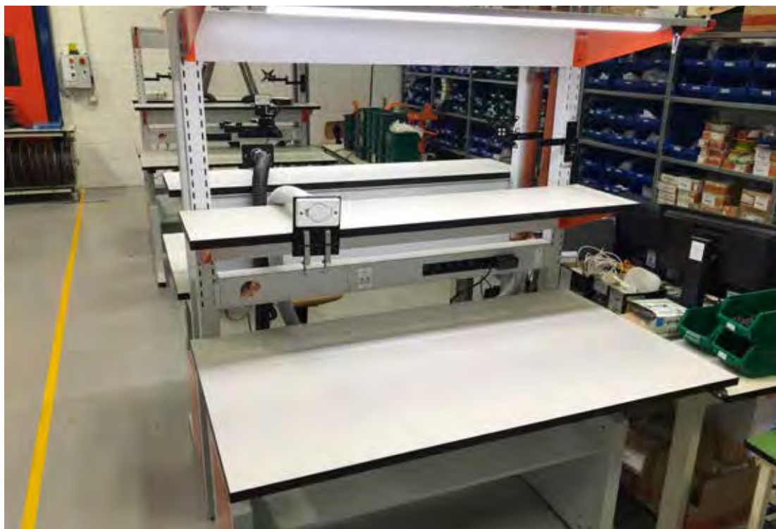
Equipped with a power bar and RJ45, bracket for extraction arm and monitor holder arm (fig.2)
