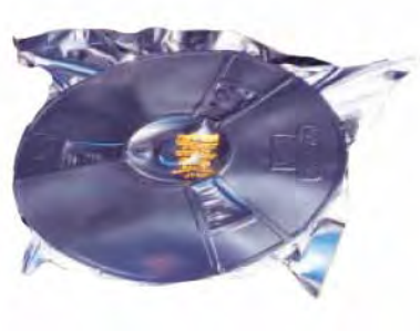
Barrier bag sealed with excessive vacuum.
