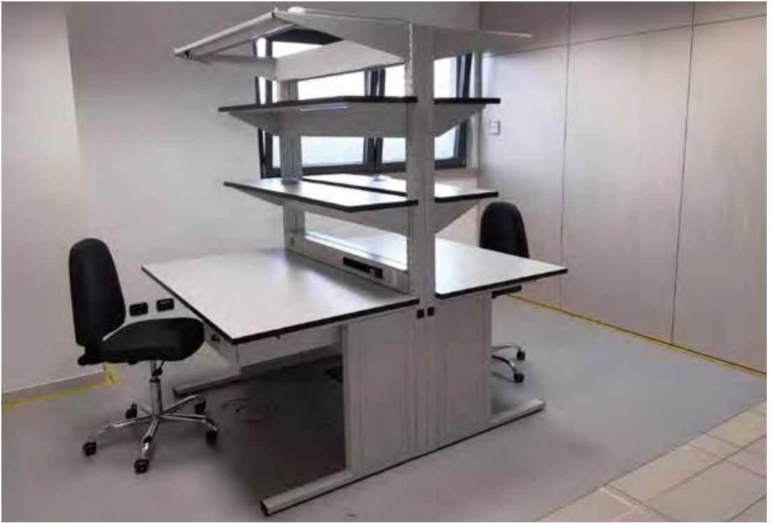
2 KE HIGH ESD-SAFE workbenches set against each other to form one unit in an EPA.
